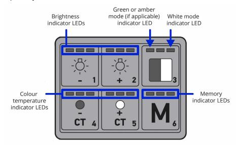
The Control Panel is working on the CAN Bus and performs data communication with the Gateway. Six buttons are available for control command inputs and 18 LEDs can indicate User and Gateway feedback messages.
