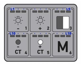
The following functions are assigned to the buttons and LED indicators of a SMART Lighting Control Panel.
